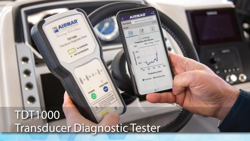
Eliminate the guesswork and guickly determine if a transducer is in proper working condition with AIRMAR's TDT1000, the first transducer diagnostic test device for use with most marine transducers. AIRMAR's SensorCheck™ App connects directly to AIRMAR's database and compares the transducer performance onboard the vessel to its original, factory-approved test results.
