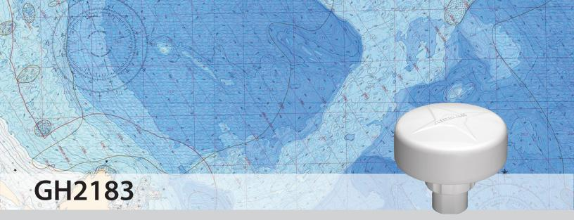
The patented Airmar GH2183 combines GPS positioning and highly accurate heading information in one compact antenna. The GH2183 eliminates the need to install a GPS antenna above deck and a heading sensor below deck. Only one above-deck installation is required, saving installation time and money. The waterproof housing protects the internal components—all of which are solid-state (no moving parts). This means the GH2183 can withstand almost any condition that exists in the marine environment.
