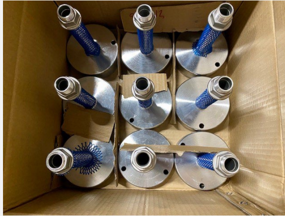
Rejected packaging: parts migrating under or around dividers
