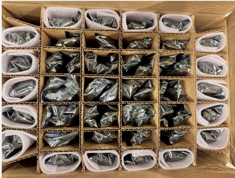
Approved ESD packaging for printed circuit boards
