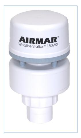
Caption: Shown above is one of the new WX Series WeatherStation® models—the 150WX—at the actual size. Airmar's WX Series instruments are the only all-in-one weather monitoring solution to offer true and apparent wind speeds without additional sensors. To ensure the accuracy of each product, every unit is factory calibrated in a wind tunnel at our state-of-the-art facility located in Milford, New Hampshire.
